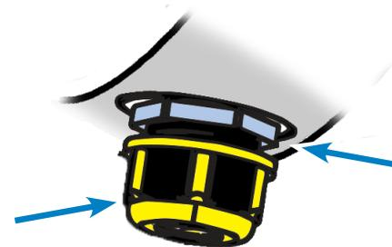
The thin nut secures the connector to the extension mount.
